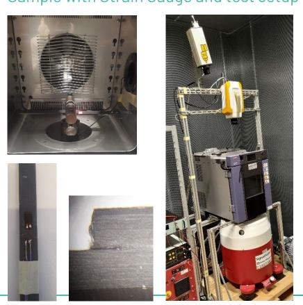
Fatigue damage growth and critical event for an IM7 sample
