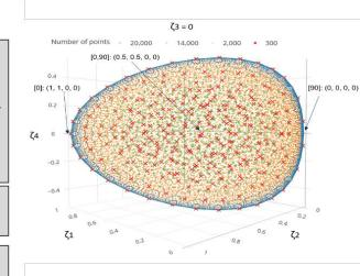
Feasible lamination parameters space (z1, z2, z3, z4). Projection with z3 = 0. Four levels of simplification (20,000 blue to 300 points - red).
